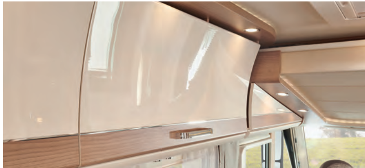
Overhead storage cabinet front panels: high gloss ivory with wooden strips and chrome piping
